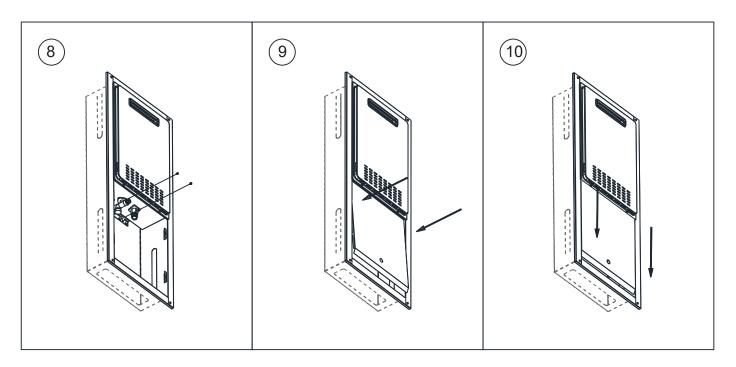
! IMPORTANT! Use a weatherproof electrical socket if necessary and weatherproof the recess box if required by using suitable sealant along the external joints and around the pipework.
